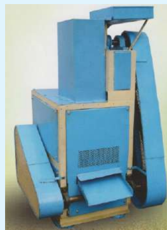
Millet de-huller cum Pearler (GB Pant university, Pantnagar)
