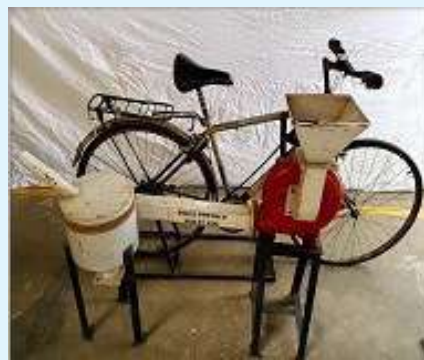
CFTRI-Pedal Operated Millet Dehuller, Capacity= 10-12 kg/h
