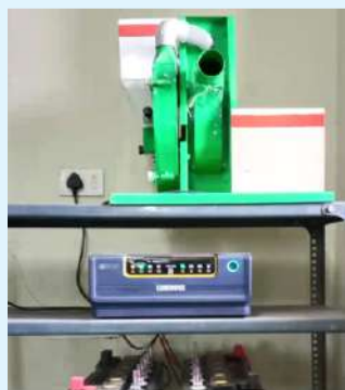
Solar Powered Small Millet Dehuller (Small Millet Foundation Funded by IIMR), Capacity= 30-80 kg/h
